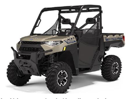
Id. ¶ 12. Each vehicle comes equipped with a roll cage, also known as a rollover protective structure or "ROPS." See Mot. at 1-5. The ROPS serves to protect occupants in the event of a rollover of the vehicle. See id.
